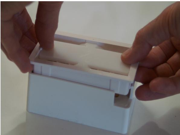
After dipping tops in Sealing Solution, the liquid capsules are joined (above). Then capsules are ejected into drying rack (left), where they are allowed to dry (below).
